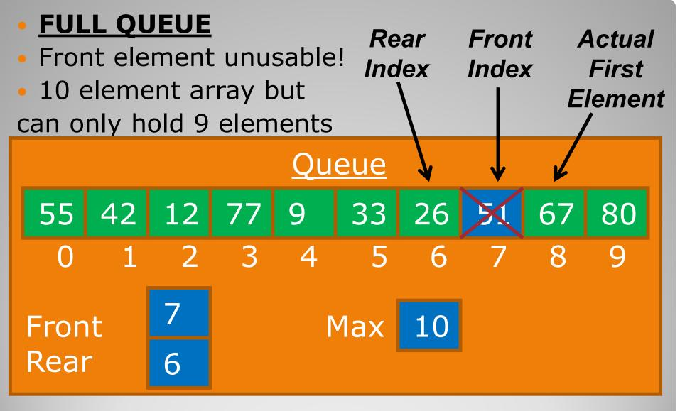
QueueArrayBased Constructor Set max to 10 Set items to new int[max] Set front to max - 1 Set rear to max - 1
