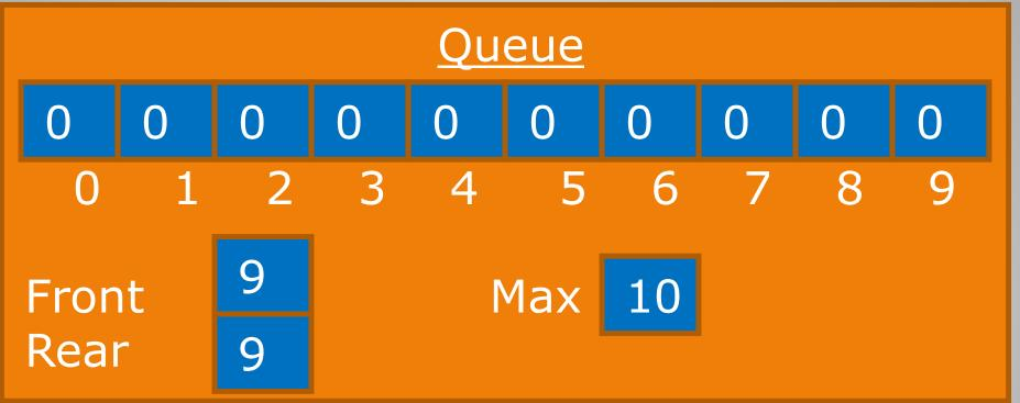
What does a queue look like internally using an array-based implementation assuming we run the following code...
